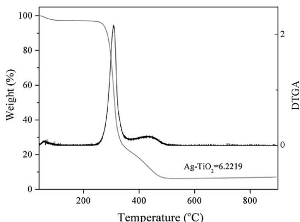
Fig. 7. Thermal degradation of Ag–TiO<sub>2</sub> covered cotton fibres under air flow; TGA (grey line) and DTGA (black line) curves of the Ag–TiO<sub>2</sub>-coated cotton fibres (ramp 5 °C/min, in air, 40–900 °C) are shown. A residual weight of about 6% has been obtained at 900 °C. This value is due to the Ag–TiO<sub>2</sub> contents in the sample.
