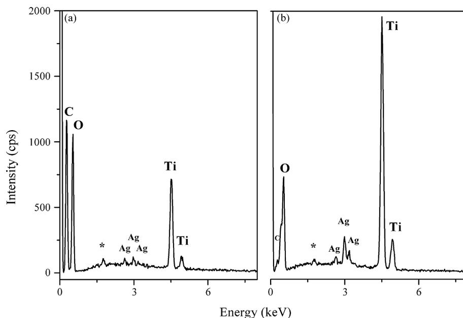
Fig. 3. EDS spectra of the Ag–TiO<sub>2</sub>-coated cotton fibres before (a) and after combustion at 500 °C for 5 h (b) (\* support).
