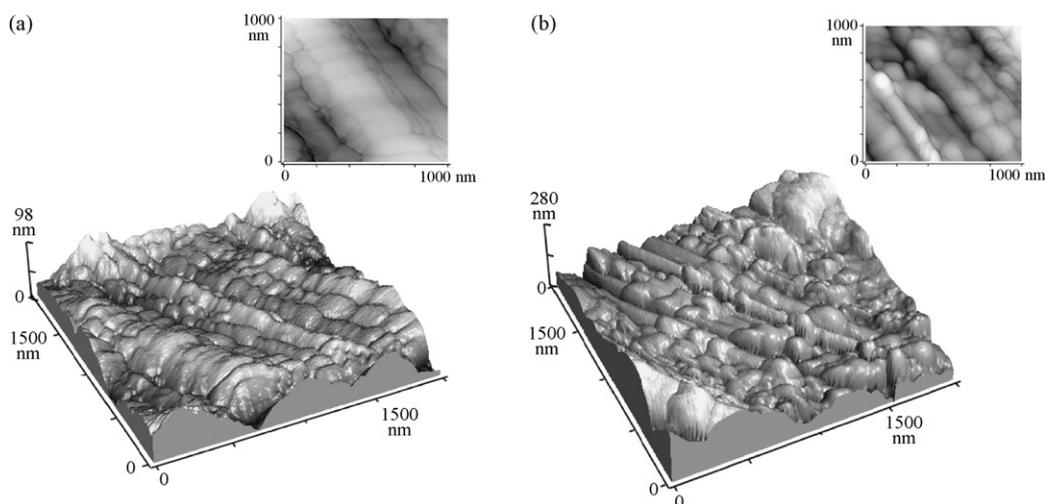
Fig. 4. (a) 3D *non-contact* AFM topographies of portion of a pure cotton fibre; (b) 3D *non-contact* AFM topographies of a Ag/TiO<sub>2</sub>-coated cotton fibre. In the insets on top 3D enlarged views of portions of the fibres are shown.
