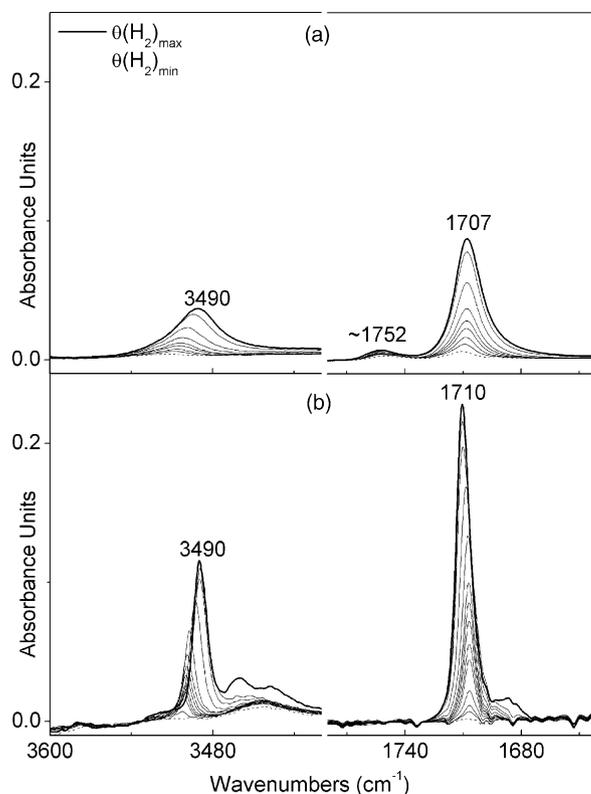
Fig. 5. FTIR spectra of  $\text{H}_2$  adsorbed at 298 K on plate-like ZnO (a) and Kadox ZnO (b) samples by decreasing progressively the coverage ( $\theta_{\text{max}}$   $p(\text{H}_2) = 16\text{ kPa}$ ;  $\theta_{\text{min}}$   $p(\text{H}_2) \rightarrow 0$ ): O–H species (on the left side) and Zn–H species (on the right side) absorption regions.
