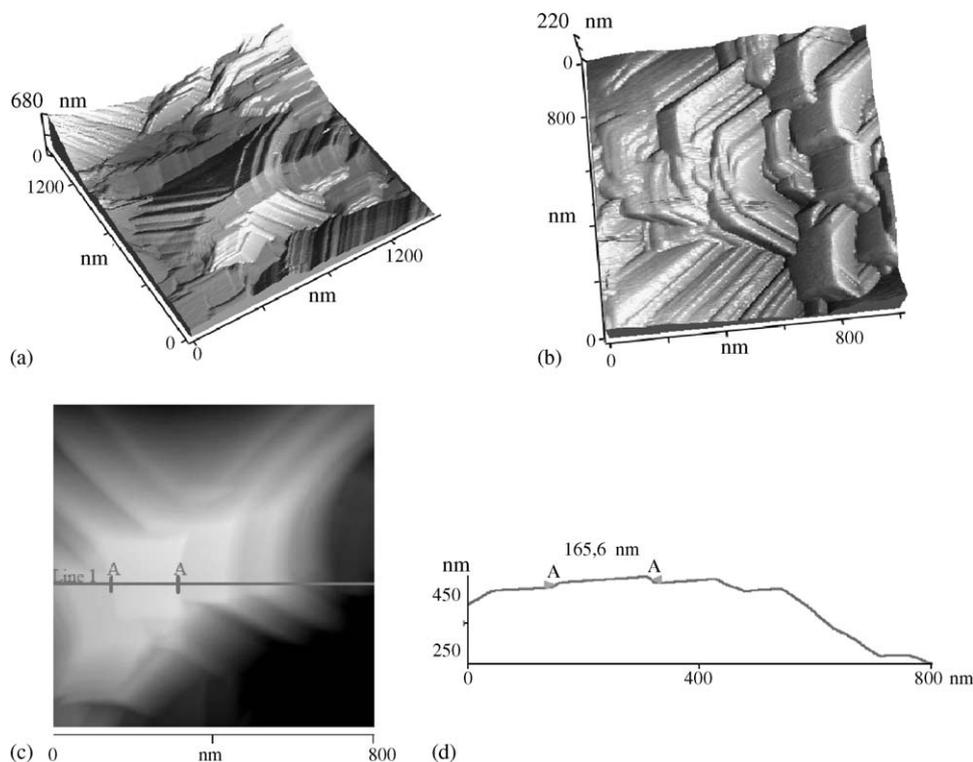
Fig. 2. Large scale contact-AFM (1.5 μm × 1.5 μm (a), 1 μm × 1 μm (b) and 0.8 μm × 0.8 μm (c)) topographies of ZnO crystallites on three different areas of the sample. (d) The height profile, measured across the grey line on the (c) image, is reported.
