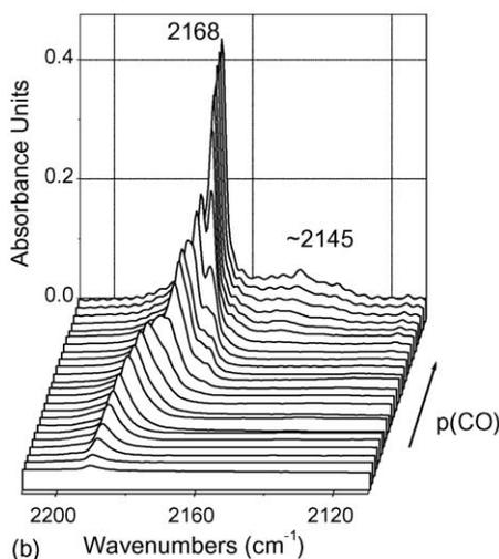
Fig. 4. FTIR spectra of CO adsorbed at 77 K on (a) plate-like ZnO and (b) Kadox ZnO samples, by decreasing progressively the coverage ( $\theta_{\max}$   $p(\text{CO}) = 2.66$  kPa;  $\theta_{\min}$   $p(\text{CO}) \rightarrow 0$ ).
